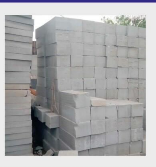
Built with Aerocon Blocks (50% less weight than generic bricks)
